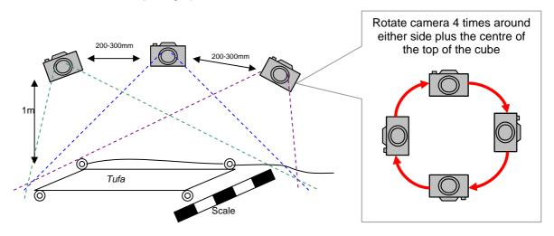
Figure 2: Camera positioning for photographing established tufa sites.
