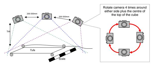
Figure 4: Camera positioning for photographing a new tufa site.
