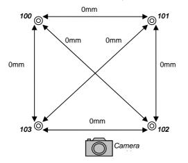
Figure 3: Measurements between each target to be taken to the nearest 10mm.
