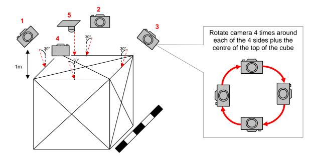
Figure 1: Camera positioning for calibration.
