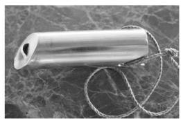
Figure 3 A hand-scraper is a 100mm long stainless steel cylinder with a single grater tooth and wrist strap. Photo: Lanyon et. al. 2010
