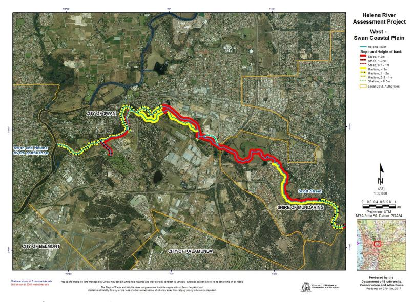
Figure 23: Slope and height of bank, West section.
