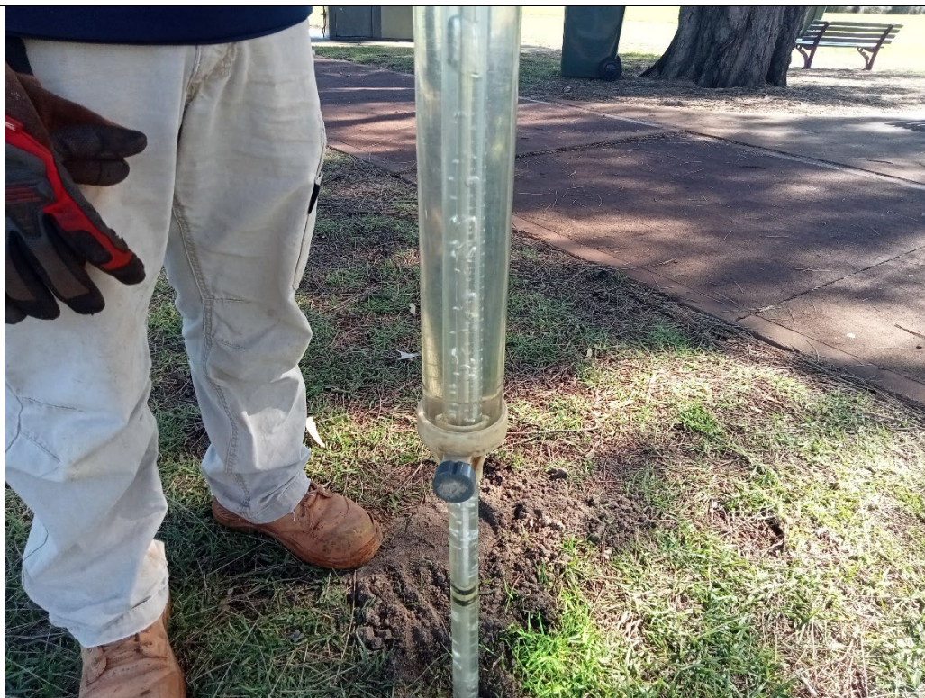
Photo 7: Infiltration test at IFT4 location.
