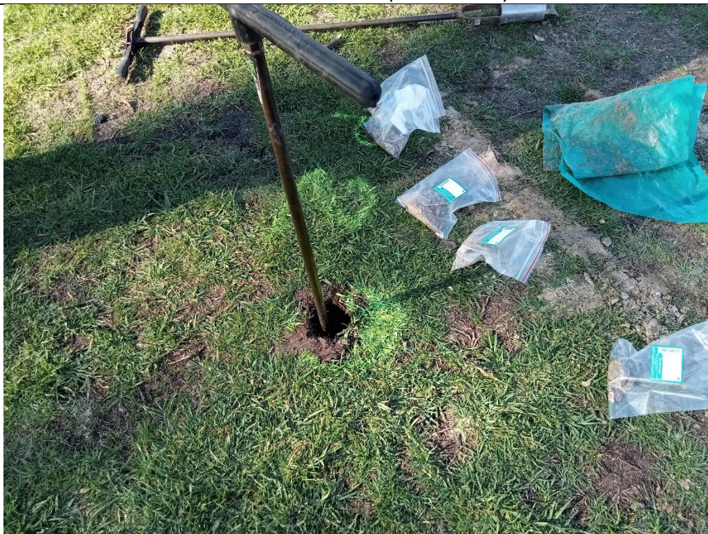
Photo 6: Environmental hand auger and sampling work at TP 2 location.
