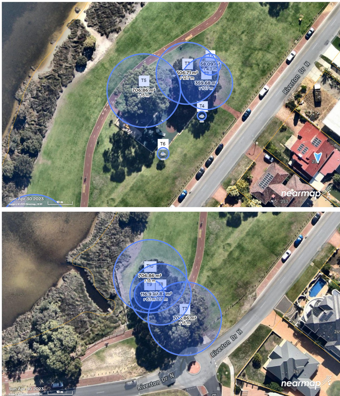
Figure 15 & 16. Tree protection zones as calculated for tree numbers 1-6 (top image) and 7-10 (bottom image). Where tree retention is desired, any excavation or construction activity within the TPZ must be root-sensitive and supervised by an AQF Level 5 Project Arborist.
