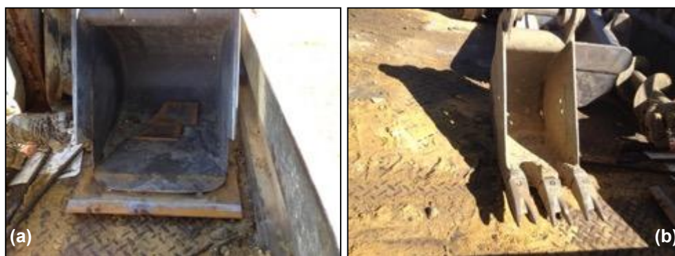
Figure 9 & 10. Where mechanical excavation is used outside the tree protection zone the selection of a toothless bucket (a) and use of a spotter can reduce tree root damage, compared with the toothed bucket (b) type which can significantly tear and damage roots for several metres.
