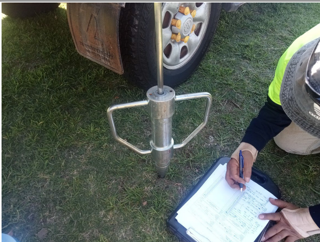
Photo 2: DCP1 test carried out adjacent to TP1 location.
