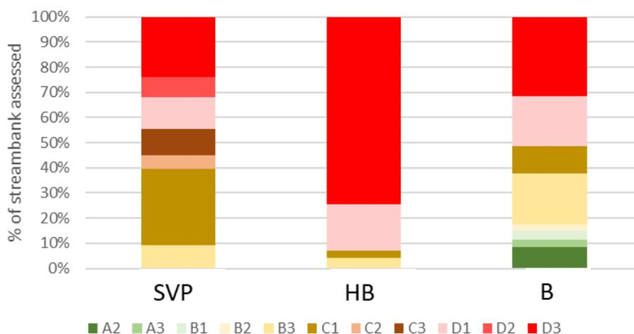
Figure 53: Pen and Scott rating for each assessment zone. Data are shown as a percentage of segment length for each zone.
