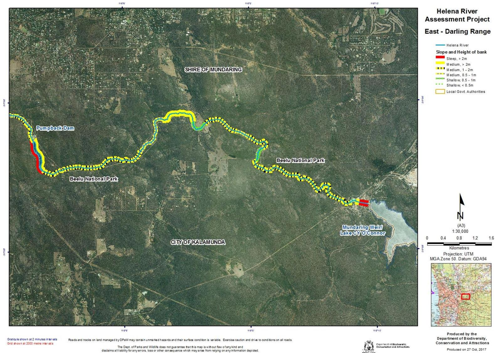
Figure 21: Slope and height of bank, East section.
