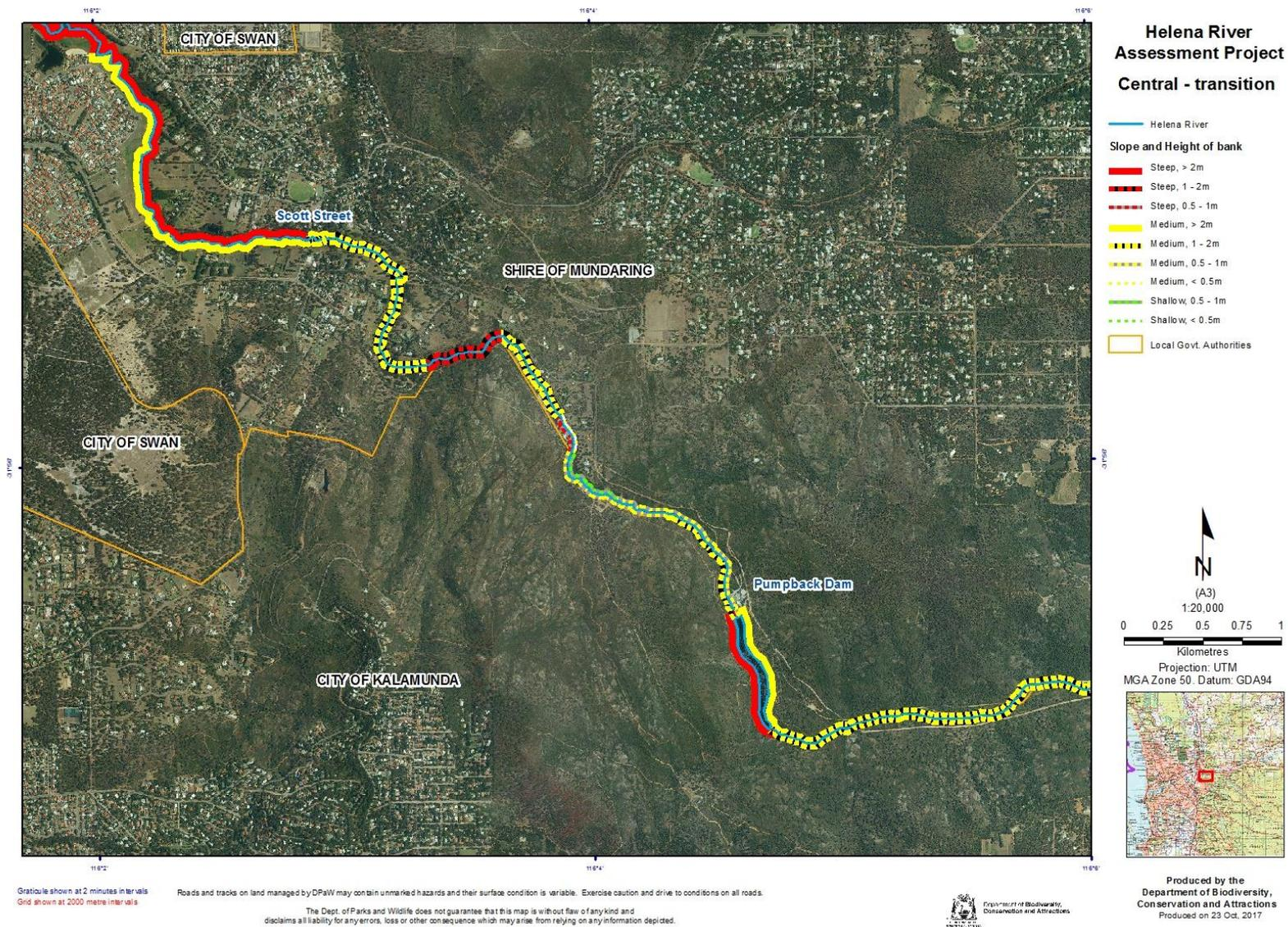
Figure 22: Slope and height of bank, Central section.
