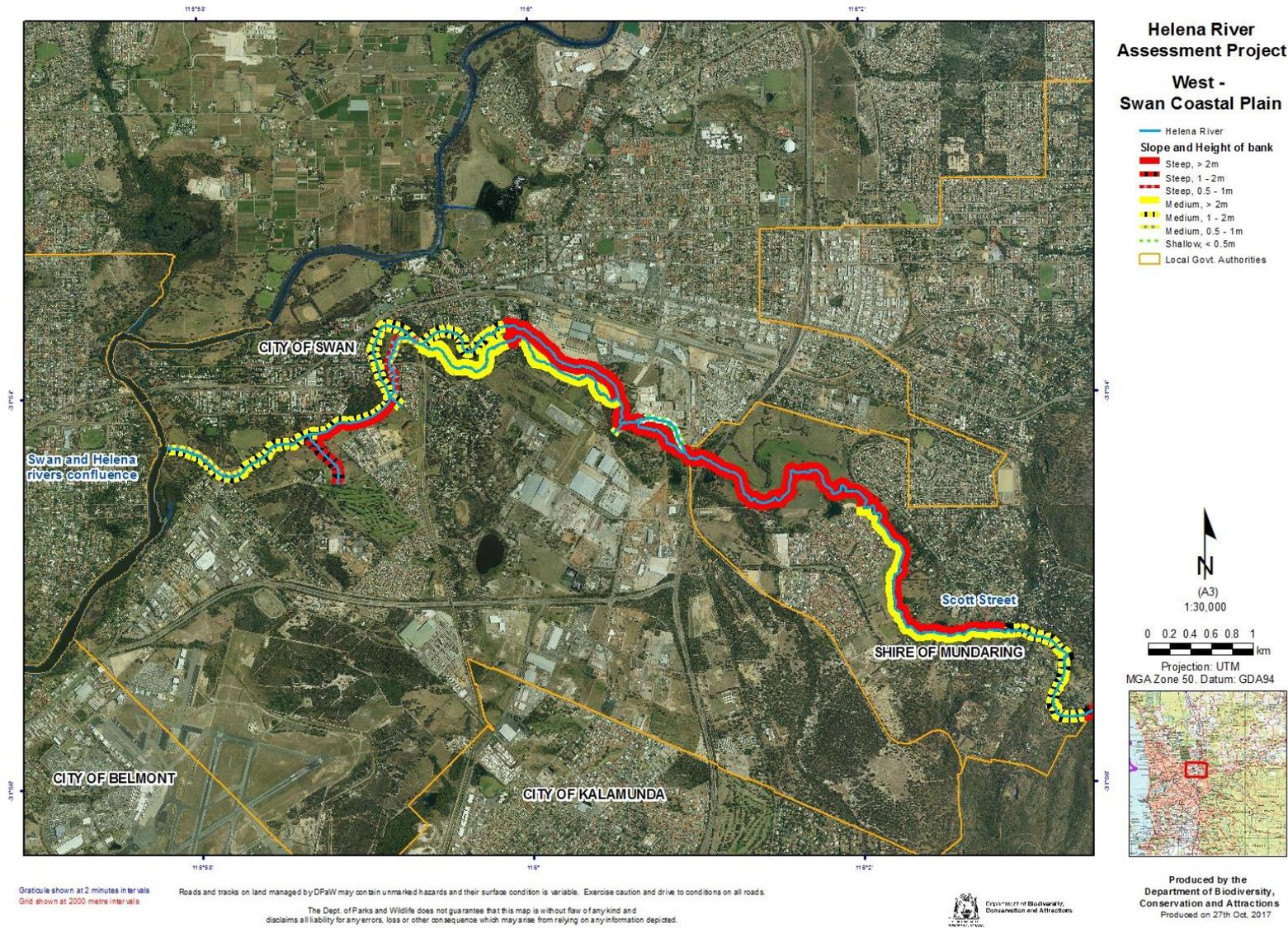
Figure 23: Slope and height of bank, West section.
