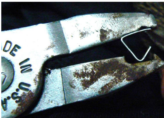
Figure 2 Set up of a metal ear tag in the pliers. Photo: Christine Freegard (DBCA)
