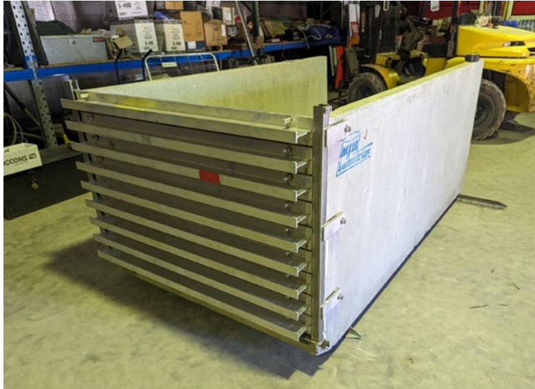
The flow control structure installed at Lower Lake Mealup involved fitting stop-boards to a concrete culvert. The stop-board frame bolts to the culvert and boards can be added/removed to achieve the desired water level.
