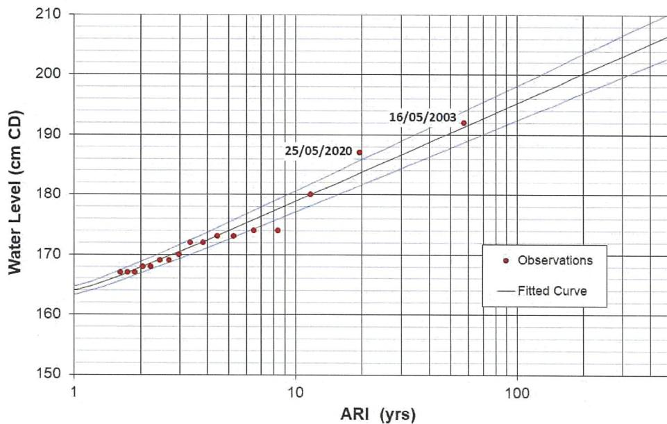
**Figure 2: Barrack Street Extreme Water Levels**
