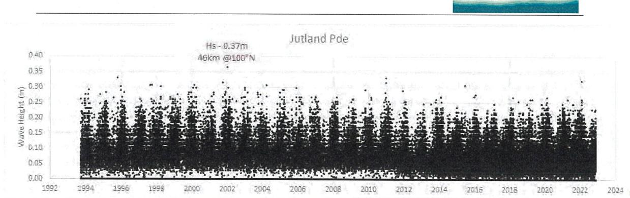
**Figure 4: Wave Hindcast from Swanbourne Wind Record**
