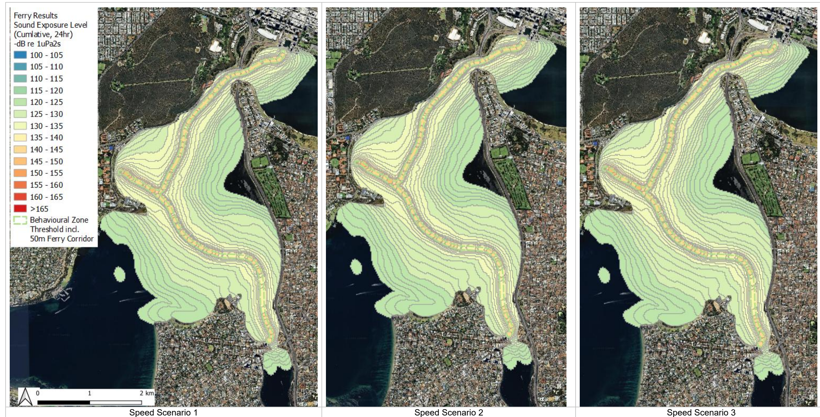
Figure C 6 Modelled noise contour plot for ferry Route 1 PCW (contours range from 120dB to 150dB)
