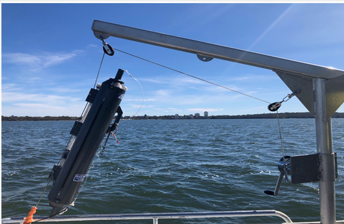
Plate 3 Niskin equivalent sampler which features a non-metallic construction with a manually activated spring closure.
