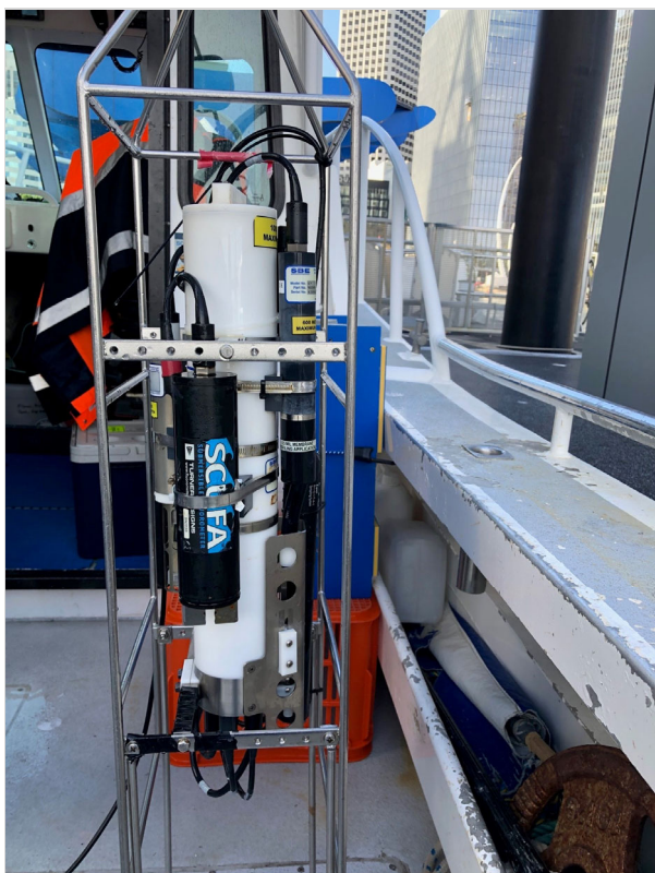
Plate 1 SeaBird (SBE) 19plus V2 SeaCAT Profiler CTD
