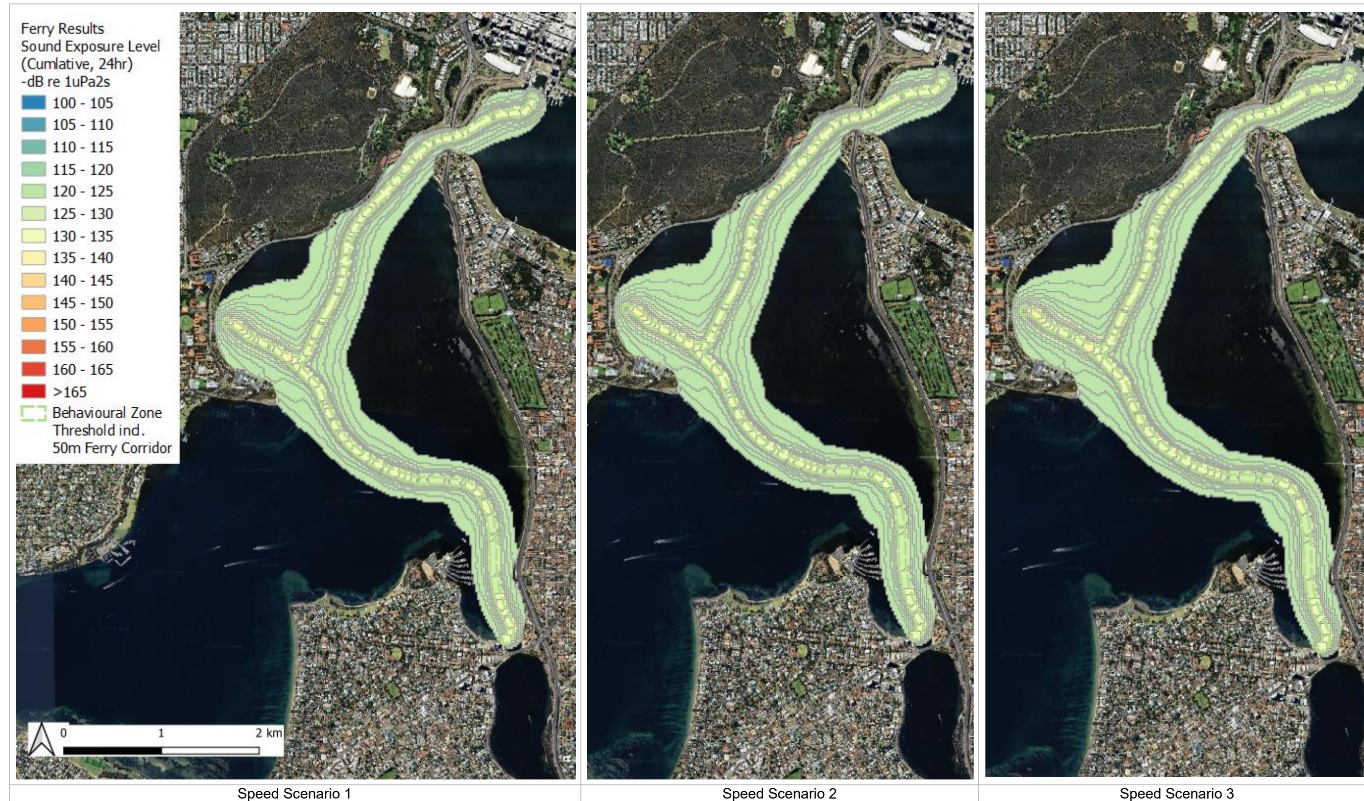
Figure C 5 Modelled noise contour plot for ferry Route 1 OCW (contours range from 120dB to 140dB)
