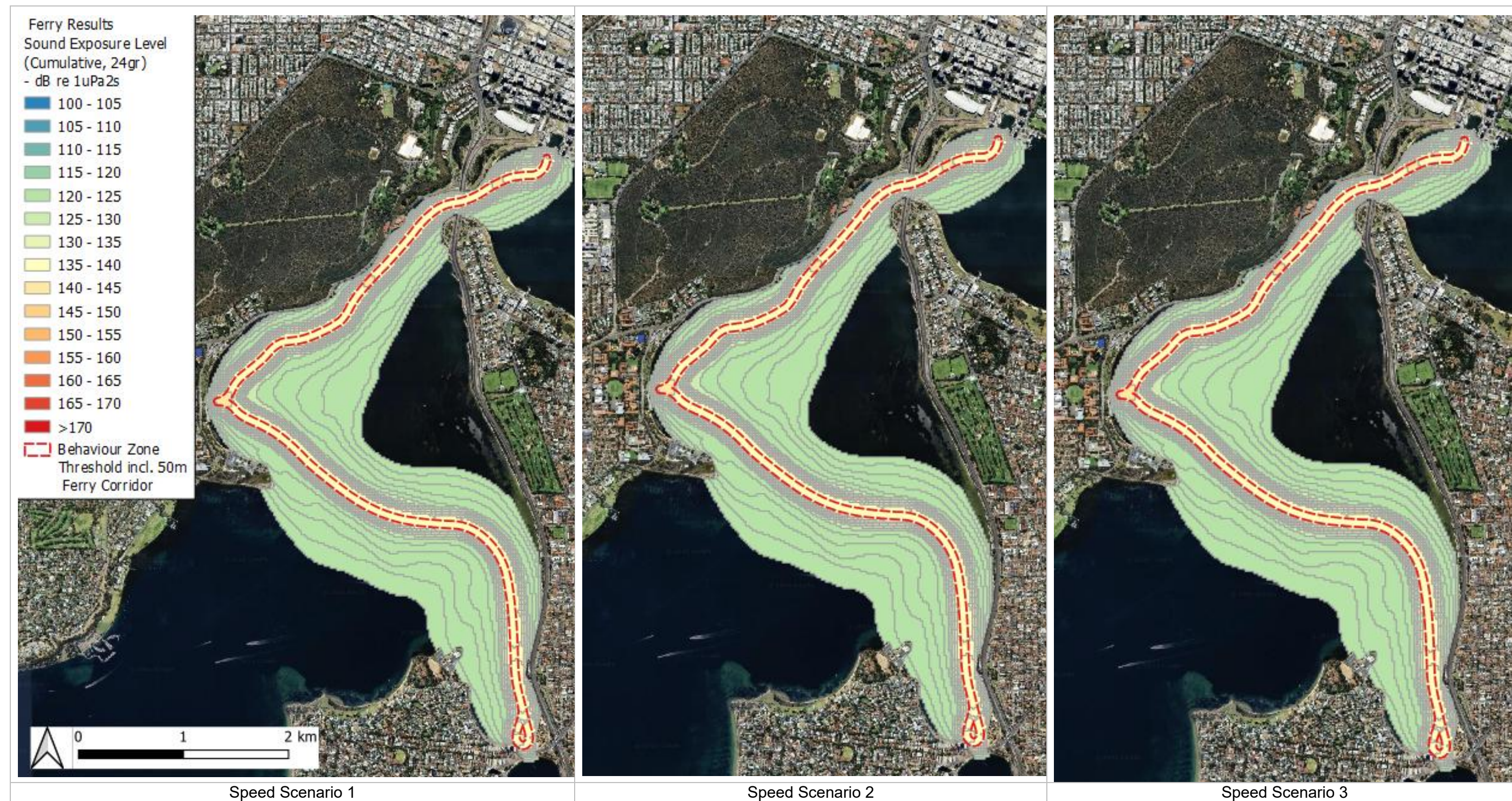
Figure C 10 Modelled noise contour plot for ferry Route 2 HF (contours range from 120dB to 145dB)
