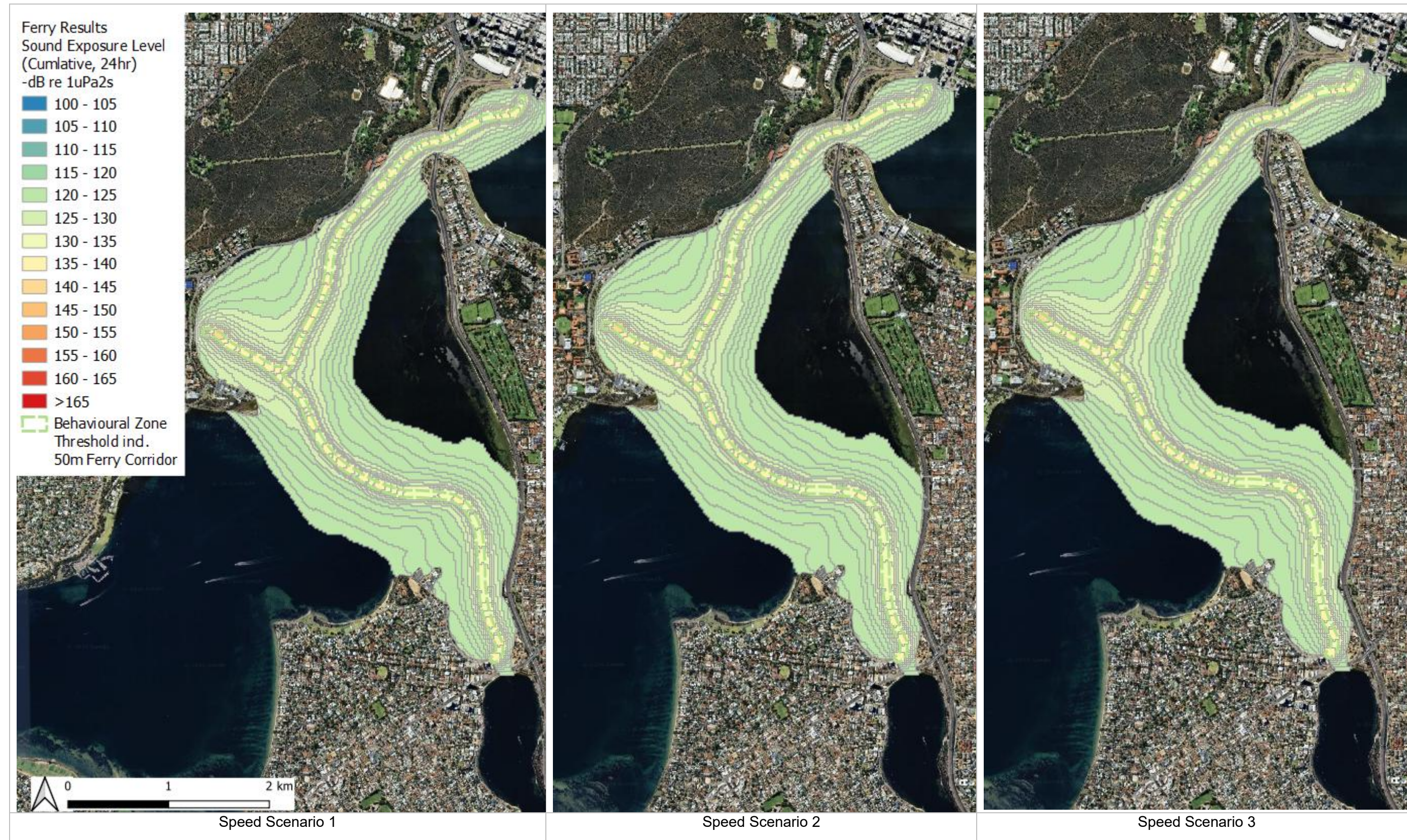
Figure C 3 Modelled noise contour plot for ferry Route 1 HF (contours range from 120dB to 145dB)
