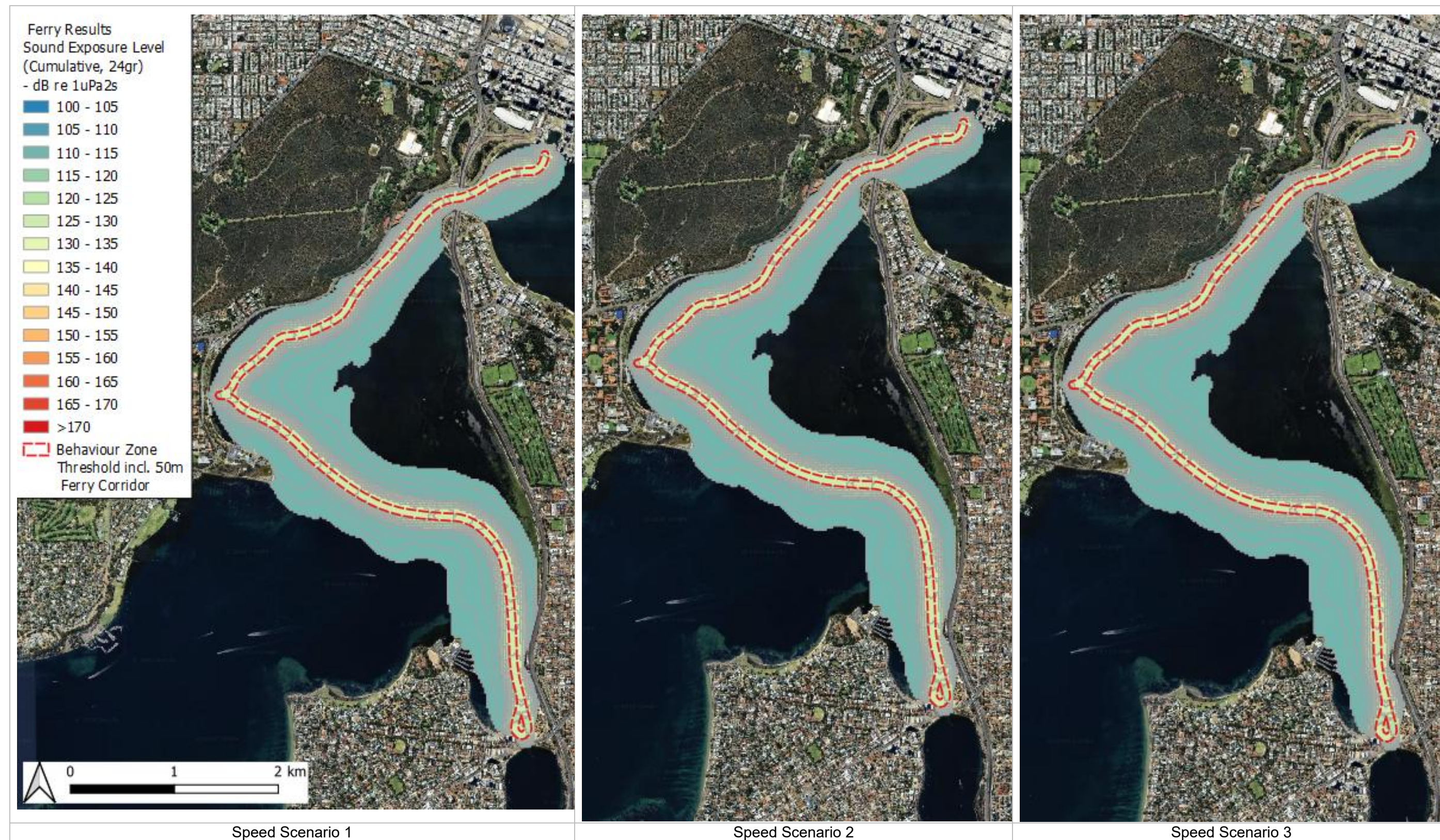
Figure C 14 Modelled noise contour plot for ferry Route 2 SI (contours range from 110dB to 130dB)
