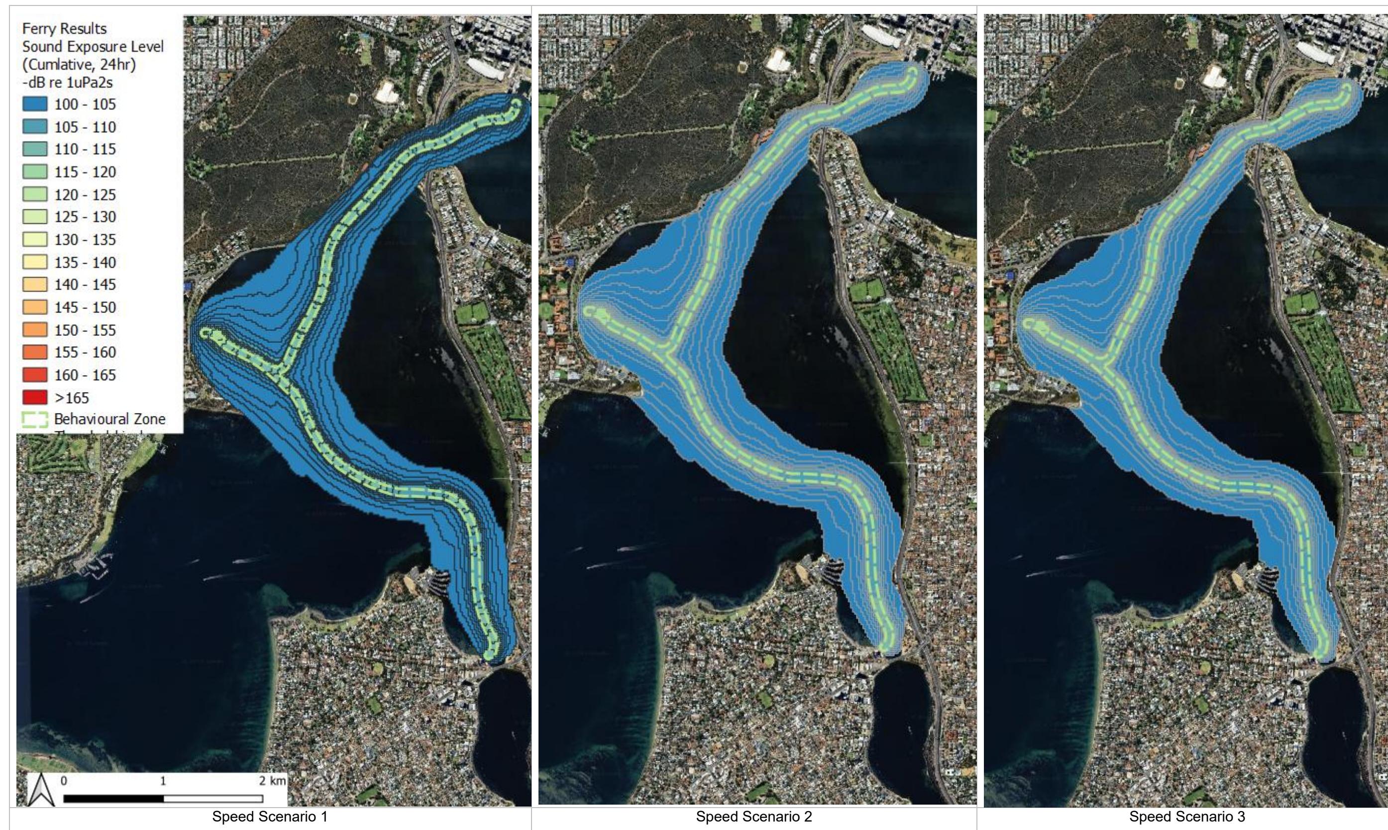
Figure C 2 Modelled noise contour plot for ferry Route 1 VHF (contours range from 100dB to 120dB)
