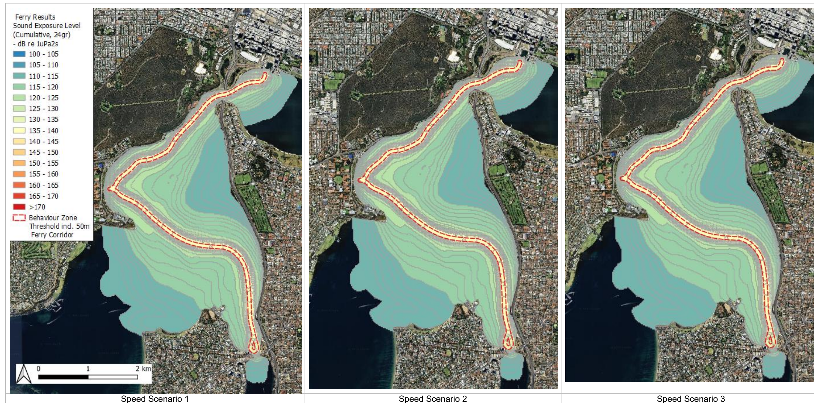
Figure C 12 Modelled noise contour plot for ferry Route 2 OCW (contours range from 110dB to 140dB)
