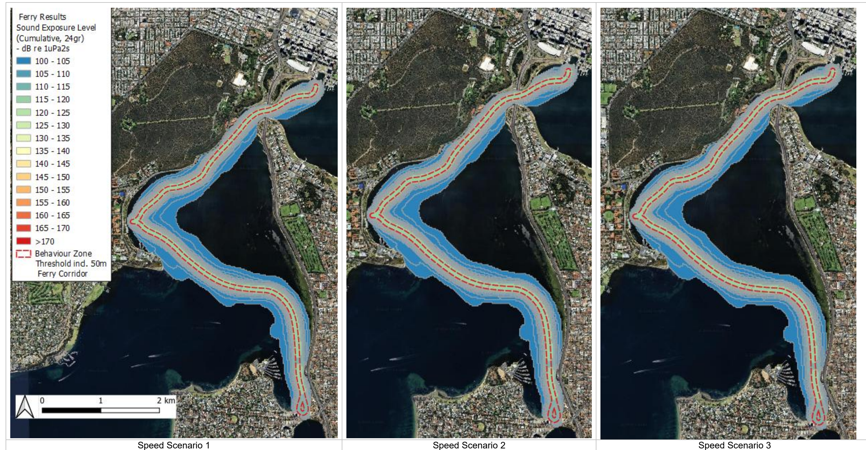
Figure C 9 Modelled noise contour plot for ferry Route 2 VHF (contours range from 100dB to 120dB)
