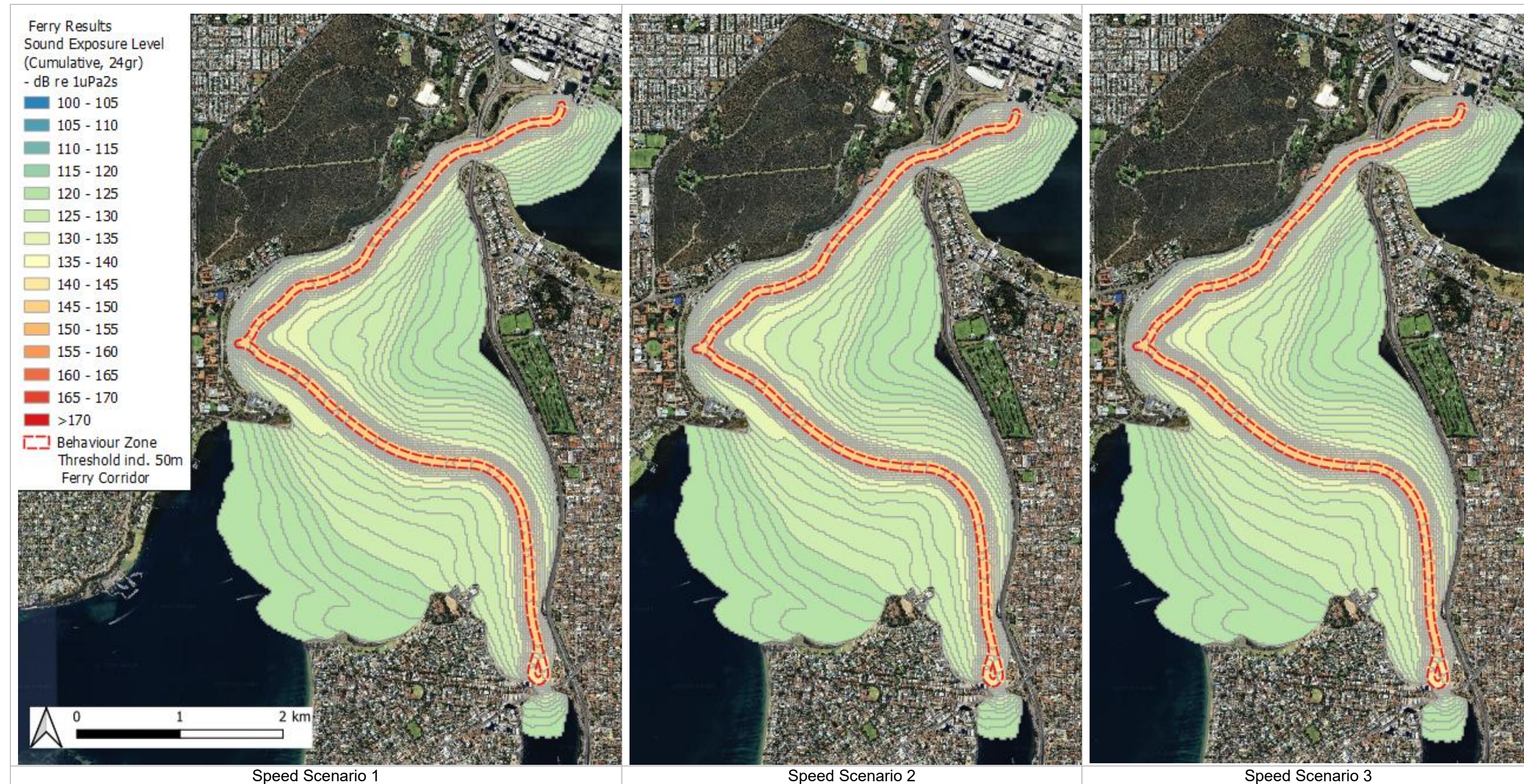
Figure C 13 Modelled noise contour plot for ferry Route 2 PCW (contours range from 120dB to 150dB)
