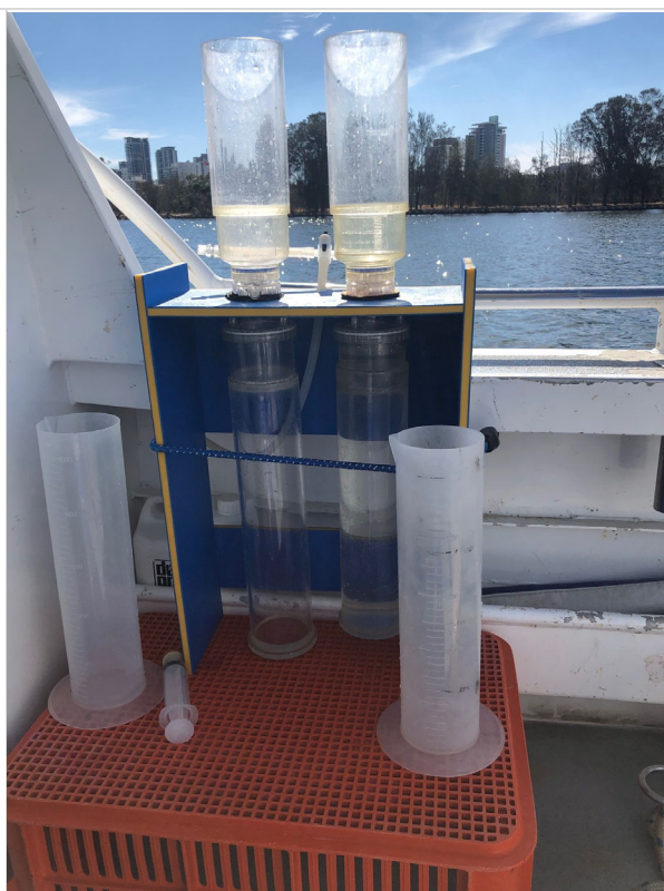
Plate 2 Field filtration equipment for algae sampling
