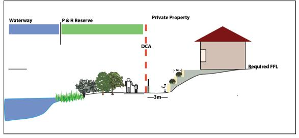
Figure 4 Terracing of retaining walls
