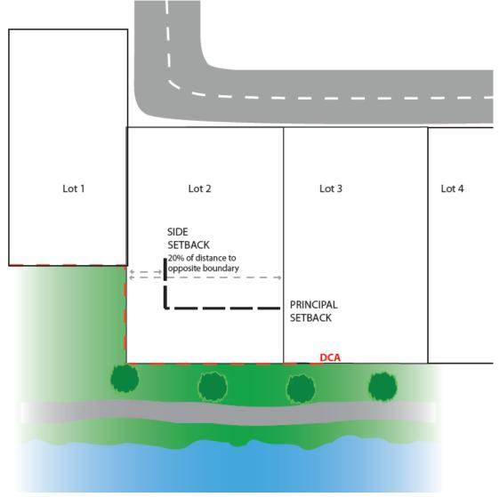
Figure 2 How to establish the side setback
