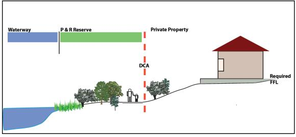
Figure 3 Graduated ground level is preferred
